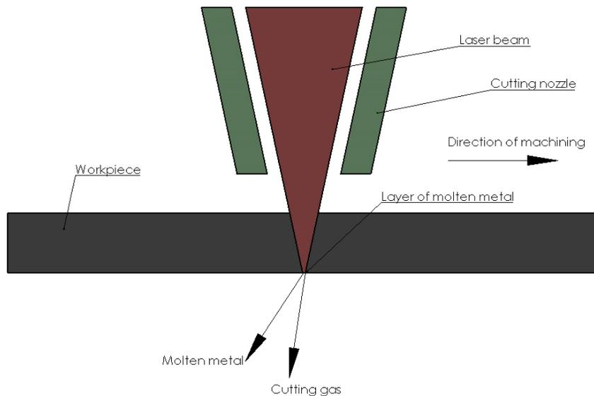
Figure 5 Describes the laser cutting procedure.
