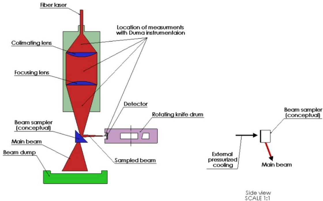
Figure 8 Schematic layout showing laser beam propagation and its measuring device
