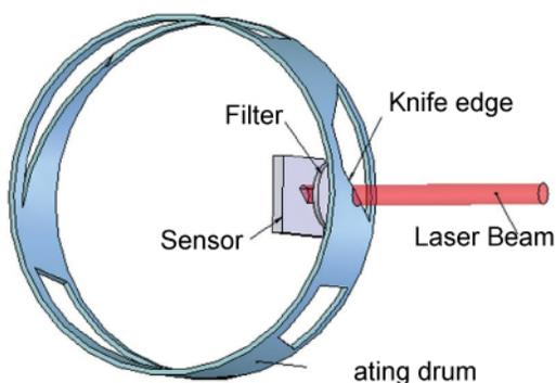
Figure 2 Simplified mechanics of a knife-edge beam profiler
